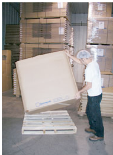
An operator sets up the 330-gal container's outer shell on a pallet. The totes hold product mixed in two stages.
