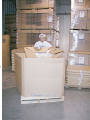
Filling the totes is quick and easy. Top, an operator opens the cassette into the shell before installing a filling-valve fitting on the liner.
