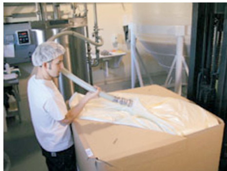
Then, the operator starts the pump for a 330-gal fill. As the liner fills from the bottom up the operator has time to go to work on other tasks.
