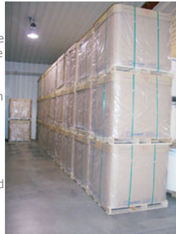
The loads are capped, shrouded and strapped and can be stacked three-high.
