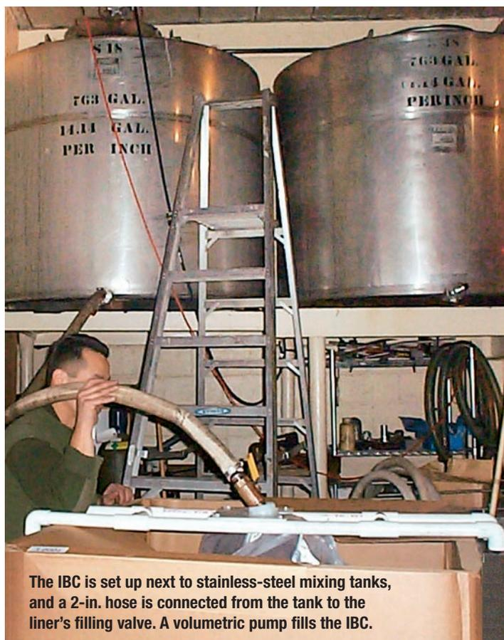
The IBC is set up next to stainless-steel mixing tanks, and a 2-in. hose is connected from the tank to the liner's filling valve. A volumetric pump fills the IBC.
